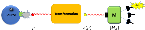
FIGURE – The basic elements of quantum information processing : preparation, transformation and measurement of a quantum system.
